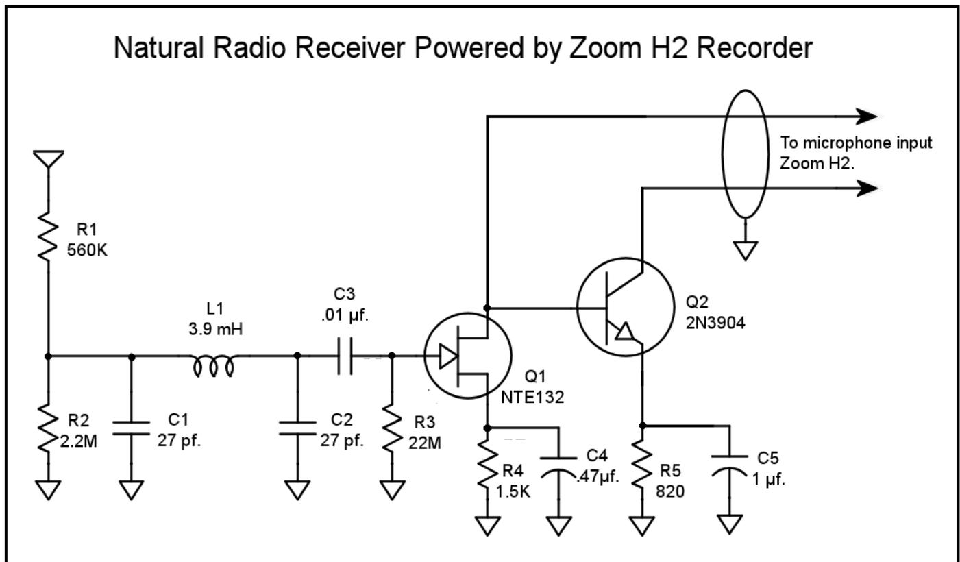
Since it appeared that the project would be viable, I refined the design a bit and added a low-pass filter to get rid of broadcast and other RF interference. With the demise of OMEGA and LORAN, the filtering is probably less necessary than it was in the past, and the filter might be able to be omitted depending on your location. Of course, if you are near one of the powerhouse Navy stations, more filtering might be necessary.
