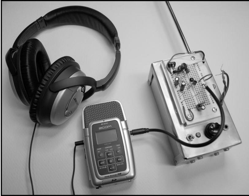
The initial tests of the breadboard unit have been encouraging. The unit seemed to have about the same sensitivity as the WR-3, which was determined in a non-scientific test while I was standing at the end of my driveway at about midnight. I heard some nice tweaks, which is about all I can ever hear in my rather poor home location.
