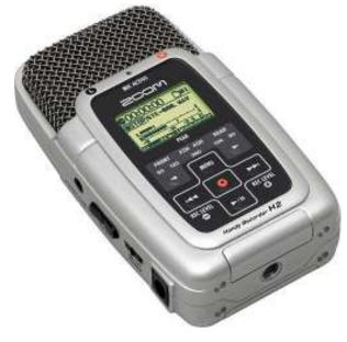
Multiple microphones are built in for a variety of polar patterns, but more importantly, there is a line input that will allow connection to your Natural Radio receiver. You can add up to a 4GB SD Card for up to six hours of stereo recording. The unit records in Records in WAV 96kHz/48kHz/44.1kHz at 16-bit or 24-bit, MP3 to 320kbps and Variable Bit Rate (VBR) data formats. The unit will record up to 4 hours on a set of AA batteries.
