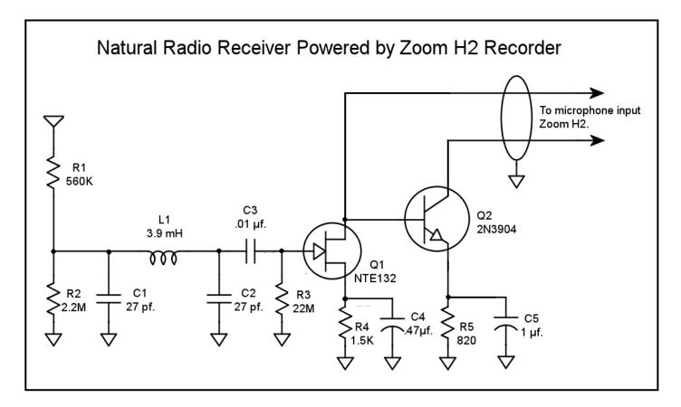
Since it appeared that the project would be viable, I refined the design a bit and added a lowpass filter to get rid of broadcast and other RF interference. With the demise of OMEGA and LORAN, the filtering is probably less necessary than it was in the past, and the filter might be able to be omitted depending on your location. Of course, if you are near one of the powerhouse Navy stations, more filtering might be necessary.
