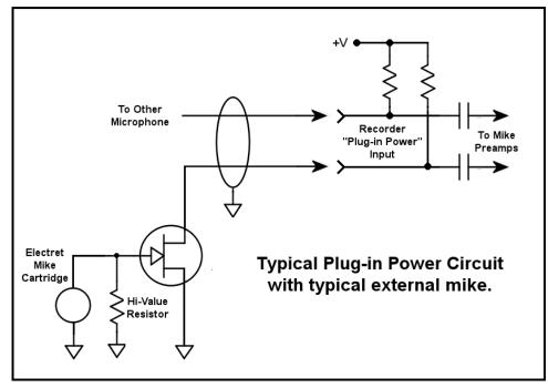
For a typical plug in mike, one of the input leads is connected to the drain of a JFET. The source is grounded and the electret's mike and a high value resistor are connected between the gate and ground. The resistor in the recorder acts as a drain resistor for the JFET and we have a preamp in the microphone powered by the recorder.
