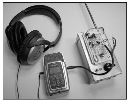
The initial tests of the breadboard unit have been encouraging. The unit seemed to have about the same sensitivity as the WR-3, which was determined in a non-scientific test while I was standing at the end of my driveway at about midnight. I heard some nice tweeks, which is about all I can ever hear in my rather poor home location.
